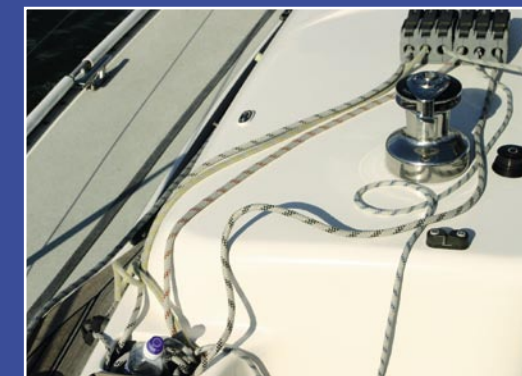
▲ Halyard-tail pockets are built into the forward ends of the coamings. Lewmar winches are standard; these are Andersen
