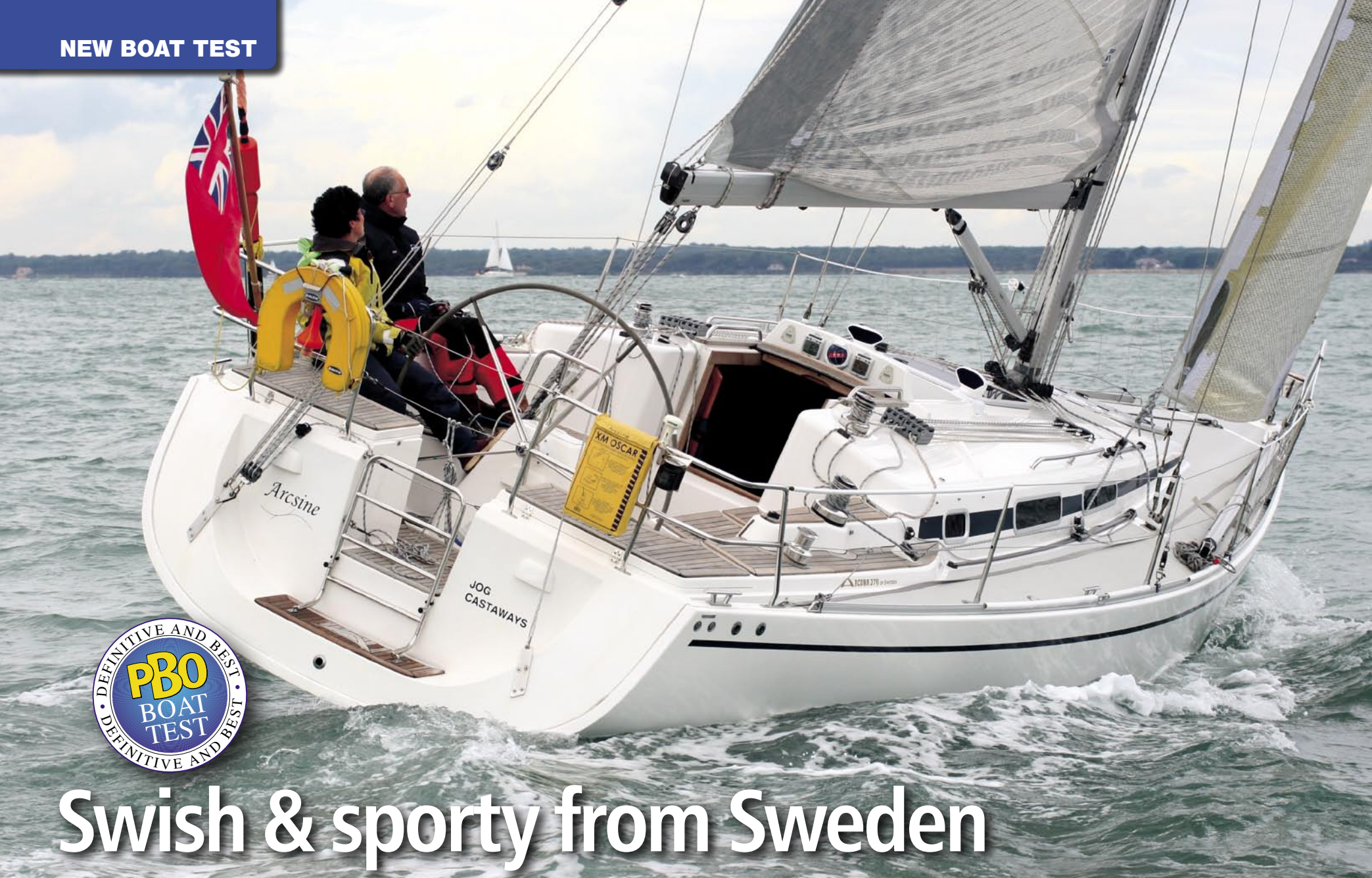
▲ The large wheel is recessed into the cockpit sole and gives the helmsman a good choice of steering positions. Winches and hardware are positioned for easy and efficient handling. A teak toerail can be fitted instead of aluminium
