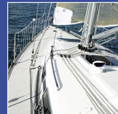
▲ Non-slip areas on deck are moulded in grey, which looks good and reduces glare but should cover more of the coachroof
