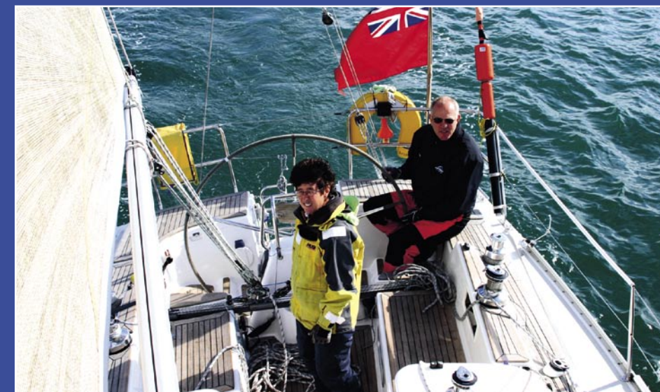
▲ The large wheel is recessed into the cockpit sole and gives the helmsman a good choice of steering positions. Winches and hardware are positioned for easy and efficient handling. A teak toerail can be fitted instead of aluminium
